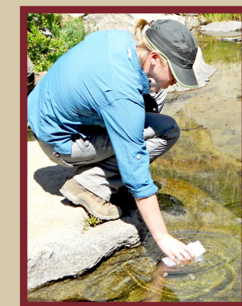
A UC Davis graduate student takes a stream water sample to monitor the effects of cattle grazing on water quality.
